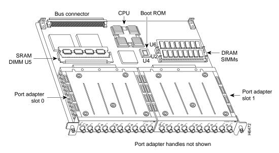
Figure 7 VIP2-15 or VIP2-40 with Two 5EFL Port Adapter Installed (Horizontal **Orientation Shown)**
